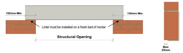
In accordance with NHBC requirements, lintels used in external walls should be installed with a separate flexible damp proof course. This should be combined with either stop ends or as an alternative the DPC should extend between 50 and 150mm beyond the end of the lintel bearing.
